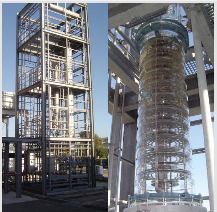
DN400 liquid / liquid extraction column, capacity 800kg/h
