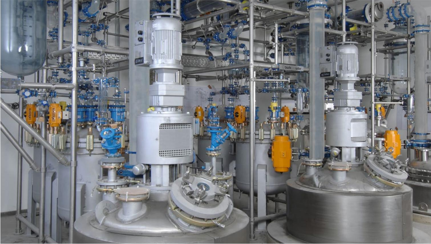
cGMP facility with 800 liter glass lined AE / BE reactors, distillation glass overhead with SiC condensers and glass lined receiver tanks for API production
