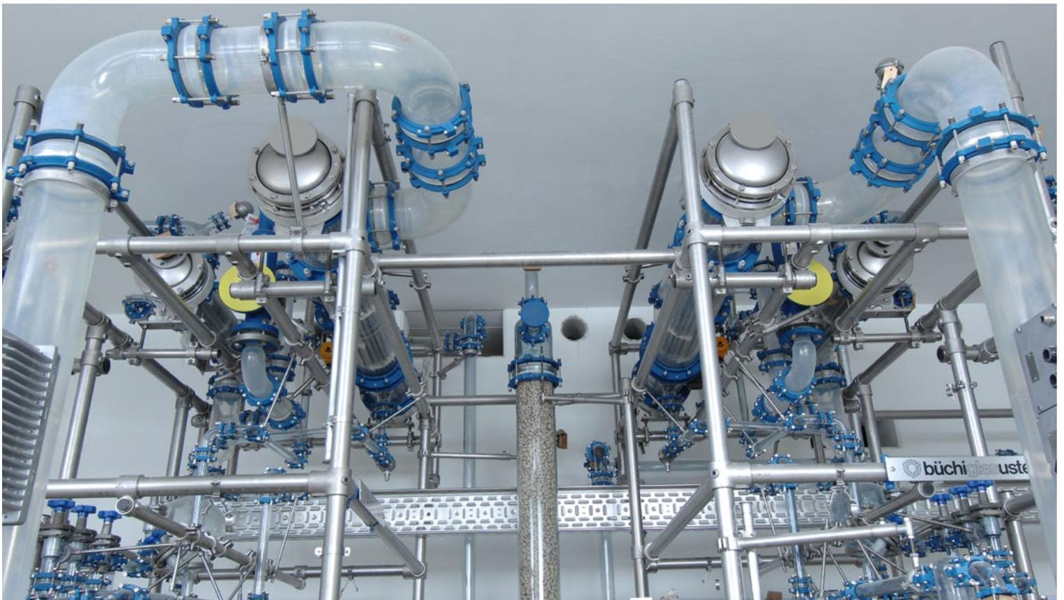
Distillation overhead with SIC shell and tube heat exchangers
