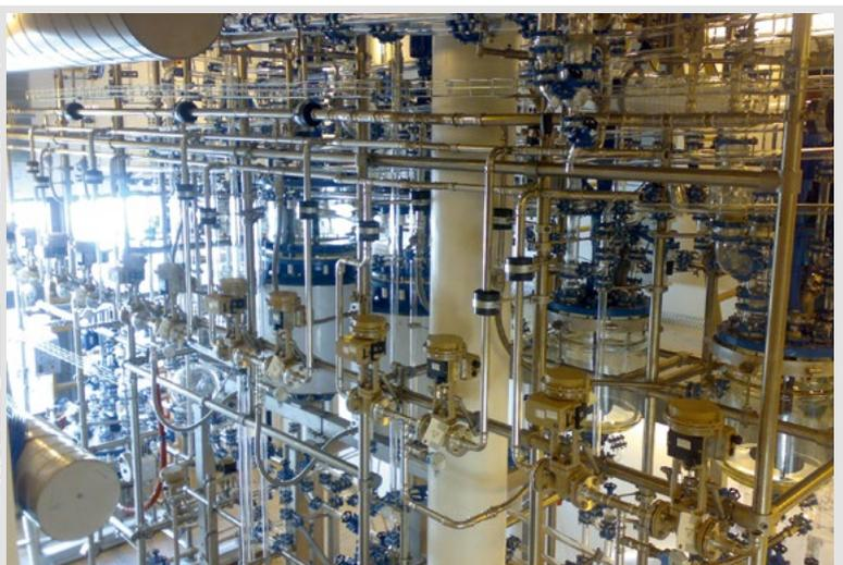
Glass tubing / piping – easy and safe due to flexible glass connection
