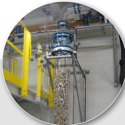
Solvent recovery, packed DN300 column, reflux condenser and controlled reflux divider
