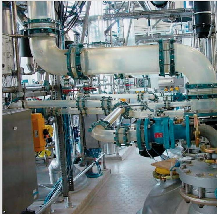
DN300 vapor line with protective glass coating
