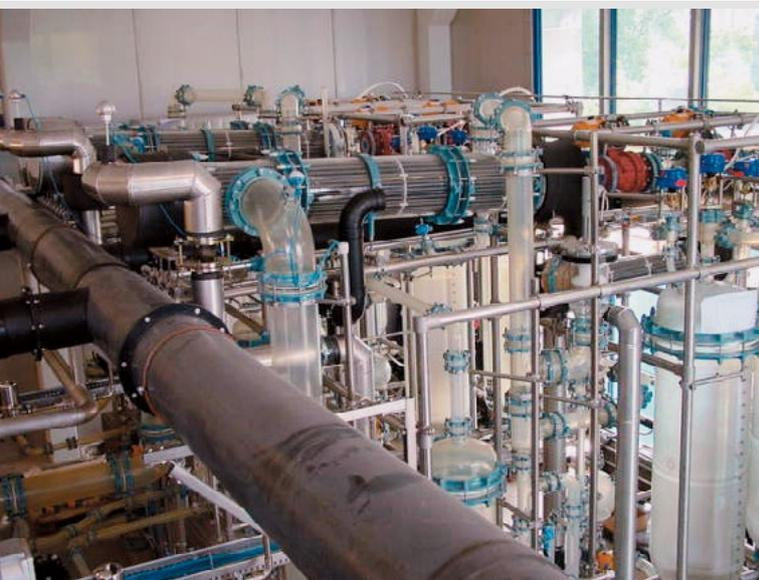
High performance SiC silicon carbide heat exchanger
