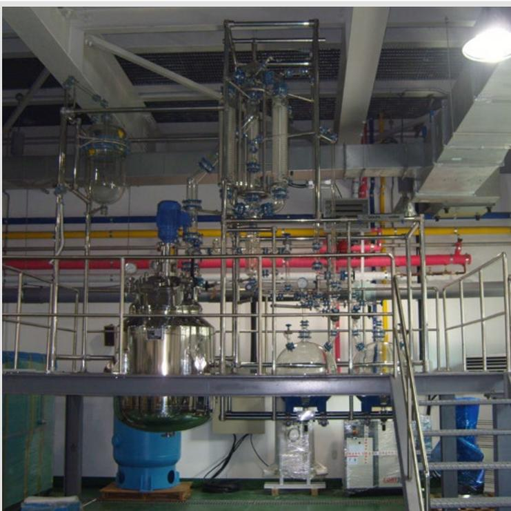
1000 liter cryogenic reactor with glass upper section
