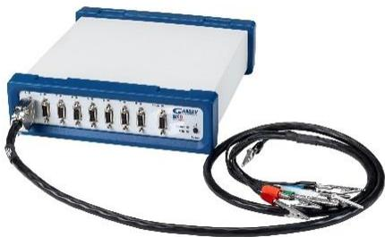
IMX8 shown with one cable. The full system comes with eight cables.
