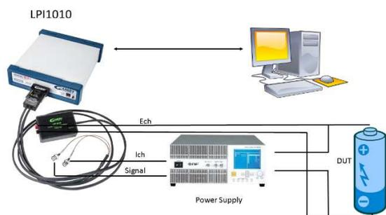
**Battery.** The measurement of  $I$  and  $E$  at a given frequency allows the calculation of the impedance.
