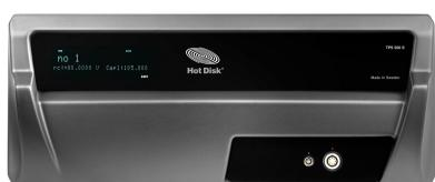
**Hot Disk instruments** with the established Transient Plane Source (TPS) method allows rapid, accurate and non-destructive testing of Thermal Conductivity, Thermal Diffusivity and Specific Heat Capacity of most material types, all in a single measurement. Optional Measuring Modules also allows to characterize anisotropic behavior of materials.
