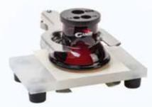
The design of the PTC1 Paint Test Cell is very simple in order to keep cost down, for most users require many cells for testing. The flat sample under test is clamped between a glass tube with an O-ring seal and the PTFE base. The tube is partly filled (20–50 mL) with the test electrolyte and sealed with a rubber stopper. A reference electrode (possibly saturated calomel) and a graphite rod counter electrode are mounted through the stopper.
