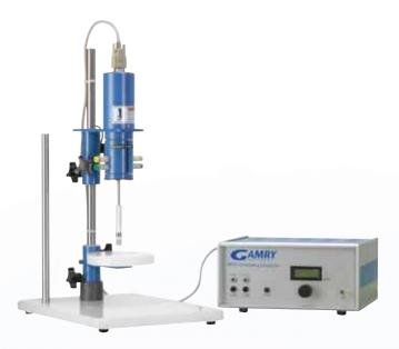
The RDE710 Rotating Electrode is a research-grade rotator and features the ability to use rotating ring-disk, disk, and cylinder electrodes. The rotation rate is adjustable from 50–10,000 rpm (revolutions per minute). The controller displays the rotation rate and is controlled by a rotation rate knob. The electrode assembly of the rotator has a versatile design that allows you to use diverse electrode types. Different shaft and electrode tips can be selected depending on your desired use.
