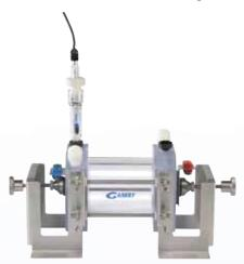
The ParaCell Electrochemical Cell Kit is designed for convenient mounting of a wide variety of flat samples. The design of the ParaCell places the working electrode and either a graphite counter electrode or a second working electrode in an opposed geometry. The cell is designed so that large and bulky samples (e.g., a 30 cm wafer) can be accommodated on either end for experiments involving two electrodes such as galvanic corrosion or electrochemical noise.
