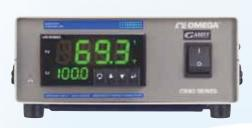
cooling sources connected to your cell are turned on and off by the TDC5 to maintain the desired temperature. The TDC5 is a closed-loop system, meaning it measures the temperature of the cell using a platinum RTD, and uses feedback to control the heater and/or
