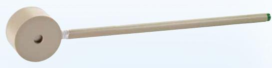
The Flat Specimen Holder is designed to hold flat, circular or square samples for use in the Multiport Corrosion Cell. This optional holder is designed to handle circular samples from 25 to 30 mm in diameter or square samples with sides of length up to 23 mm. The actual exposed electrode face is 10 mm in diameter with an area of 0.785 cm<sup>2</sup>. Samples can be up to 7 mm thick.
