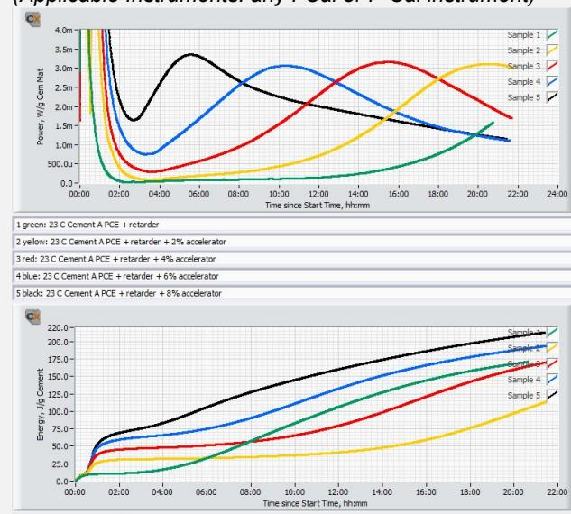
Shotcrete accelerators work through accelerated formation of calcium aluminate sulfate hydrates. The reactivity of the aluminate and sulfate phases in the binder used is of particular importance, both of which are visible in isothermal calorimetry, making it an excellent tool for optimizing admixtures for shotcrete as well as for the selection of binders for shotcrete.
