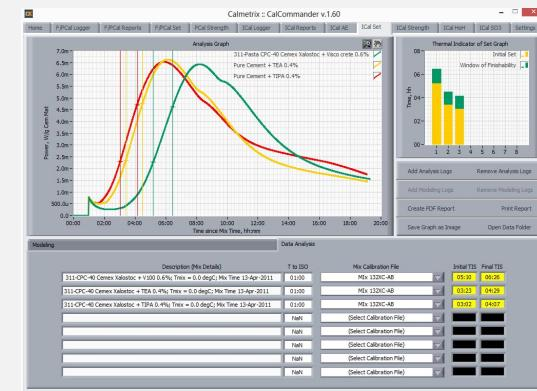
Isothermal calorimetry can be used to estimate setting times, as heat rates shown in the Power curve correlate with physical test data obtained applying a standard such as, for example, ASTM C403.
