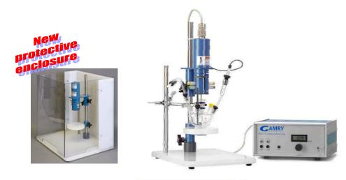
The RDE 710 Rotator is a solid state controlled servo-system that is the preferred electrode rotator for use in the research laboratory. Rotated Disk (RDE), Rotated Ring-Disk (RRDE) and Rotating Cyclinder Electrodes (RCE) may be used with the rotator. Electrode connections are made to the electrode by silver carbon brushes - two each for the disk and the ring - to provide consistent, reliable contact.
