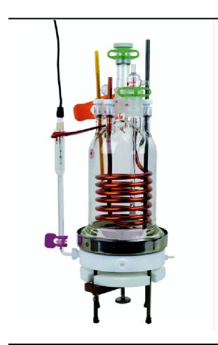
The Gamry Instruments  $Flexcell^{TM}$  is a versatile electrochemical cell designed to counteract a problem that plagues most cells -- crevice corrosion around the specimen seal. First popularized by Avesta Steel, the cell utilizes a flooded gasket seal design to inhibit crevice corrosion between the sample and its holder. This simple yet elegant design results in an easy to use, reliable, crevice-free system.
