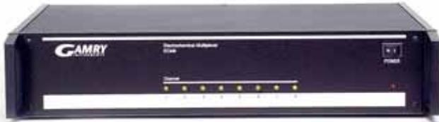
The Gamry ECM8™ Electrochemical Multiplexer is designed for electrochemical applications. The ECM8 Multiplexer connects up to eight electrochemical cells to one Gamry Potentiostat/Galvanostat/ZRA. This converts a single Potentiostat into a powerful instrument capable of automated sequential electrochemical experiments. Applications for the ECM8 include corrosion inhibitor testing, EIS evaluation of paints and coatings, monitoring of field
