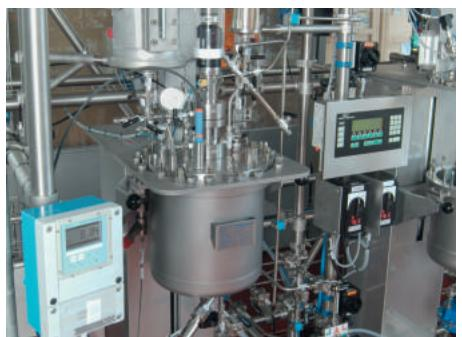
Control of suspension-polymerisation
