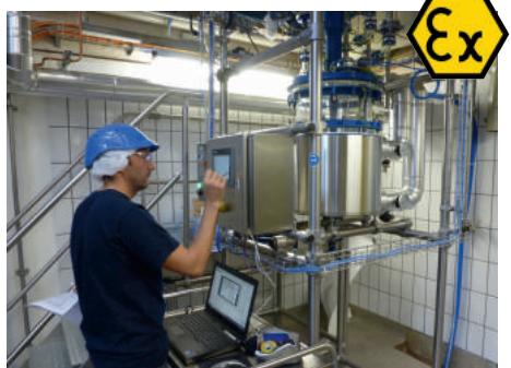
100 liter chemReactor with ATEX PLC control system
