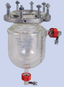
Type 1I Glass vessel with heating jacket and vacuum insulation jacket, without drain valve 0.5 / 1.0 / 1.6 / 2.0 l max. 12 bar / 200°C
