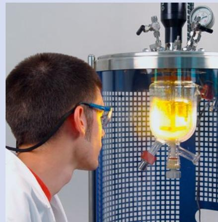
Hydrogenation in glass pressure reactor / Hydrierung in Glasdruckreaktor
