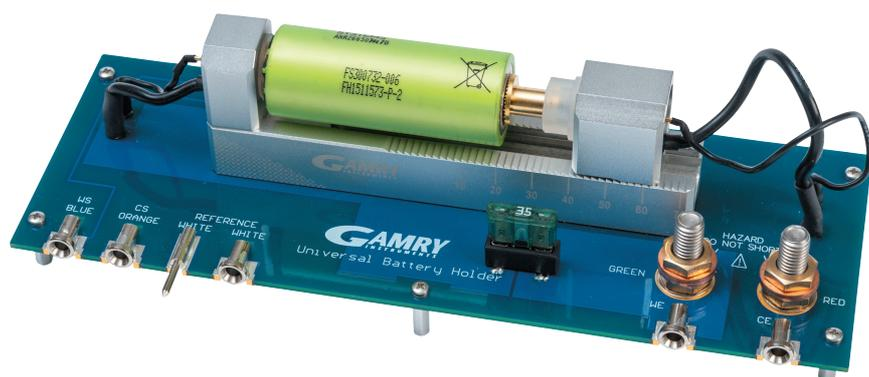
The Universal Battery Holder allows connection of a large variety of batteries, from coin-sized to larger cylindrical shapes (up to 26650), to Gamry Instruments' potentiostats. High currents, up to 30A, may be passed through the battery holder, without danger of destroying the holder. The Universal Battery Holder allows four-point measurements, and is usable with all Gamry Instruments potentiostats, including the 30k Booster.
