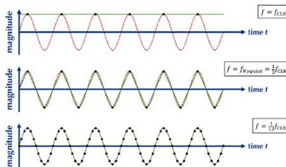
**Figure 2.** Influence of clock frequency on waveform generation.
