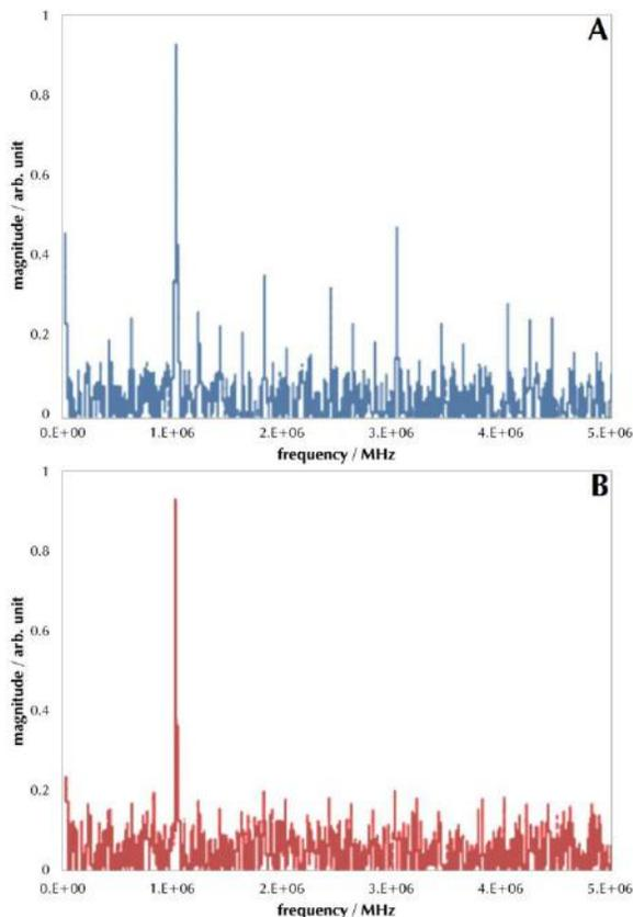
**Figure 6.** FFT of sine wave output signal shown in Figure 5. (A) unfiltered signal, (B) filtered signal. For details, see text.
