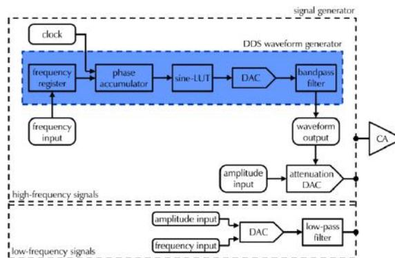
**Figure 3.** Simplified diagram of a signal generator showing both frequency-dependent methods to generate a sine wave. For details, see text.
