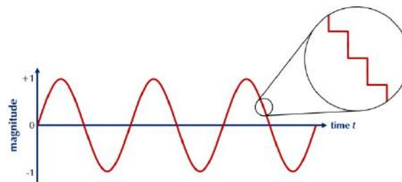
**Figure 1.** Graphical representation of a sine wave showing its digitized staircase form in greater detail.
