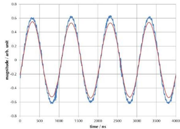
**Figure 5.** Sine wave output of an Interface 5000 before (blue) and after filtering (red).
