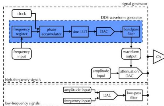
**Figure 3.** Simplified diagram of a signal generator showing both frequency-dependent methods to generate a sine wave. For details, see text.
