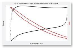
Understanding ion intercalation is an important part of battery development. Assemble your half-cell on a coated crystal and monitor mass changes as your cycle the potential – giving you insight into various charge transfer steps. Repeated cycling can allow you to understand trapping mechanisms and how they shorten device lifetime.
