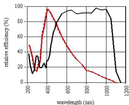
Figure 5 – Efficiency curve: 2400 g/mm. Red dashed curve: P-plane; solid black curve: S-plane.
