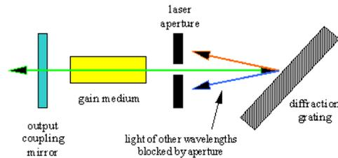
**Figure 3** – Littman tuning using a grating near grazing incidence.
