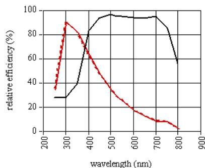
Figure 6 – Efficiency curve: 1800 g/mm, for several incidence angles  $\alpha$ .
