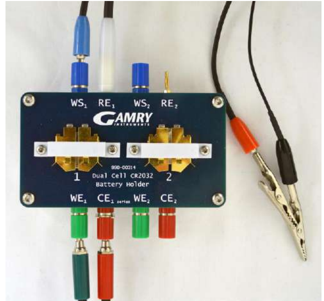
Figure 4. Dual Cell CR2032 Battery Holder with coin cells in both positions, and connections made to position 1 with cell cable.
