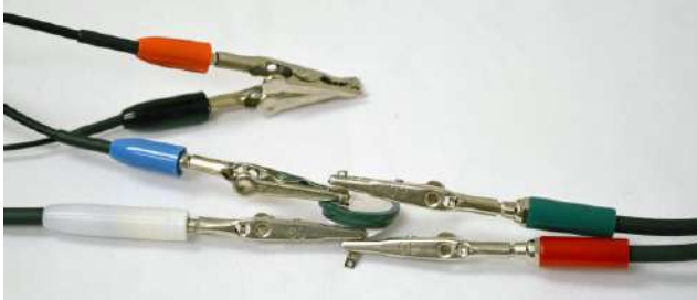
Figure 2. Coin cell with terminal tabs connected to Interface 5000 cell cables. Black and orange leads are connected together near the top of the photograph.
