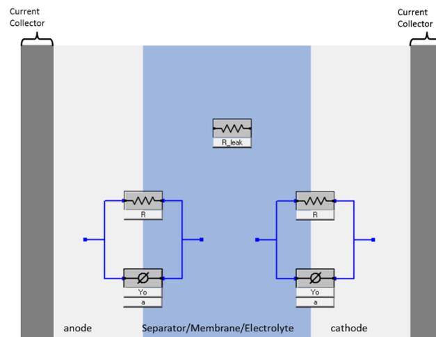
**Figure 2.** Sketch of physical model of Li-ion cell, with suggested electronic components corresponding to various parts of the cell.
