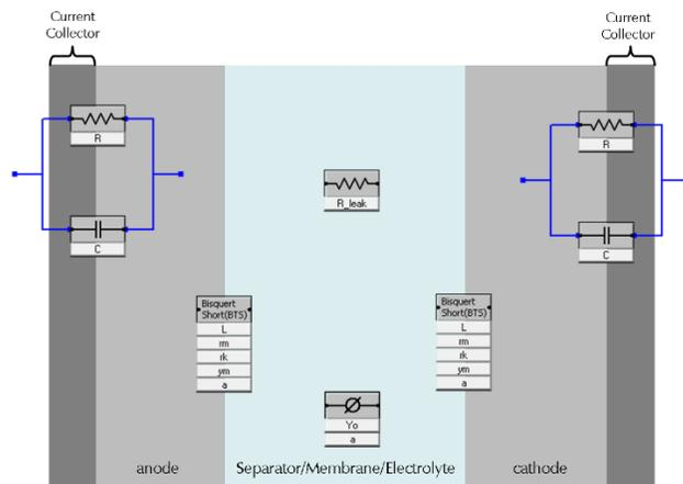
**Figure 6.** Revised physical model of a Li-ion cell, with circuit elements superimposed.
