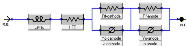
**Figure 3.** First iteration of an equivalent circuit to a Li-ion cell.
