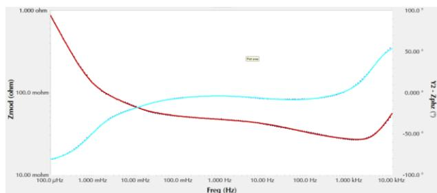
**Figure 8.** Bode plot of Li-ion data, plus fit using the equivalent circuit in Fig. 7.
