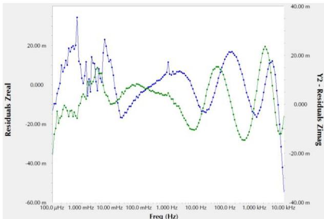
**Figure 9.** Residuals from fit to Li-ion data using the equivalent circuit in Fig. 7.
