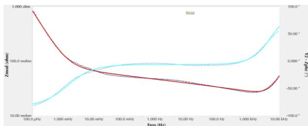
**Figure 4.** Fit using the equivalent circuit shown in Fig. 3 on Li-ion cell data.
