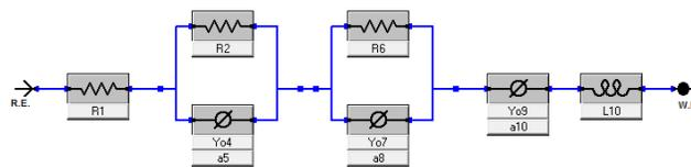
**Figure 11.** Alternate model for Li-ion battery EIS.
