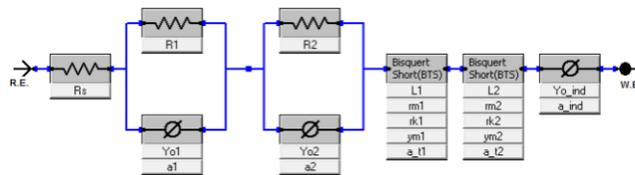
**Figure 7.** Equivalent circuit used to model the Li-ion physical system in Fig. 6.
