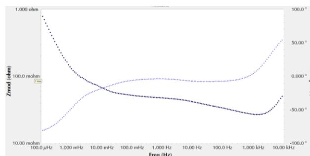
**Figure 1.** Bode plot of EIS of a Li-ion cell.
