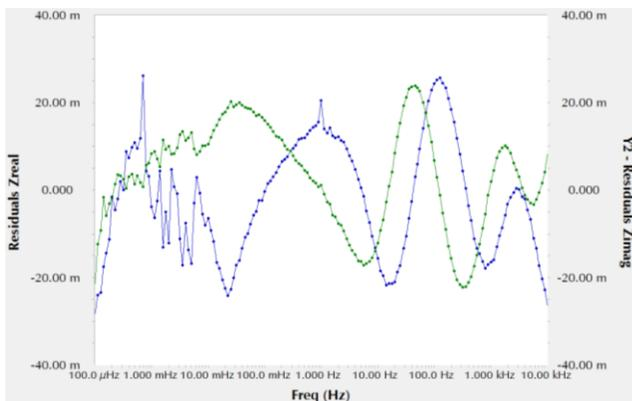
**Figure 10.** Residuals plot for equivalent circuit in Fig. 7 plus a stray inductance in series.
