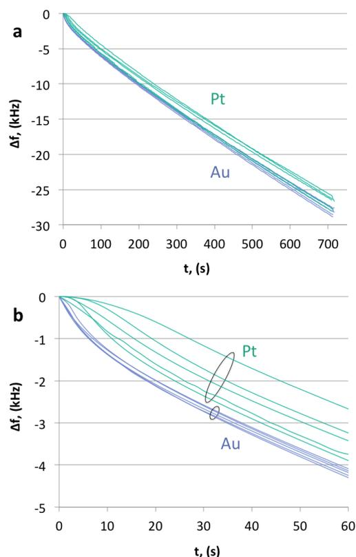
**Figure 1.** Frequency decrease recorded during (a) the entire 714 s, and (b) initial 60 s of galvanostatic deposition of PEDOT(PSS) films onto the Pt (green) and Au (blue) electrodes on the surface of the resonating quartz crystals ( $N = 5$  for each substrate). The black ovals in (b) are meant to group together the Pt and Au transients, also highlighting the differences in the reproducibility<sup>4</sup>.
