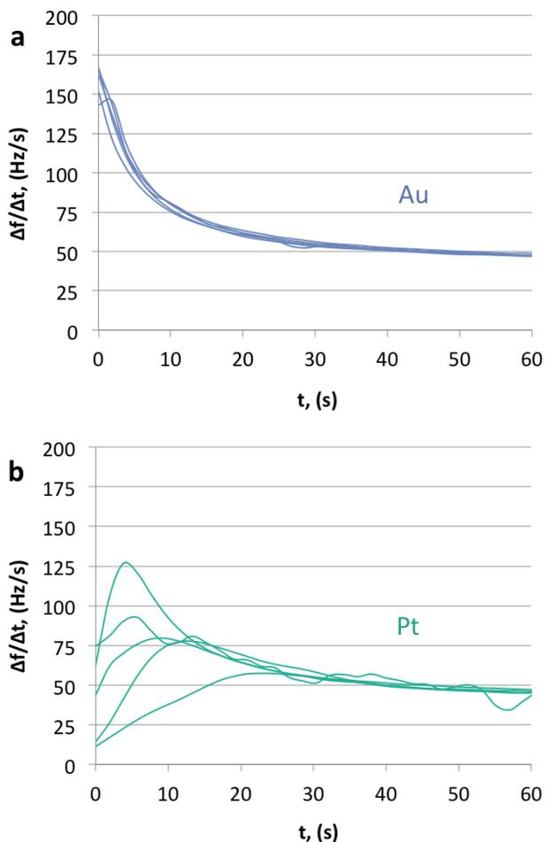
**Figure 2.** Rate change of frequency during the first 60 s of PEDOT(PSS) polymerization over Au (a) or Pt (b) electrodes on the surface of the quartz crystals<sup>1</sup>.
