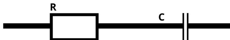
The model includes a resistor (due primarily to the electrolyte) and the coating capacitance in series.
