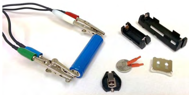
Figure 1. Selection of battery connectors for cylindrical batteries and coin cells.
