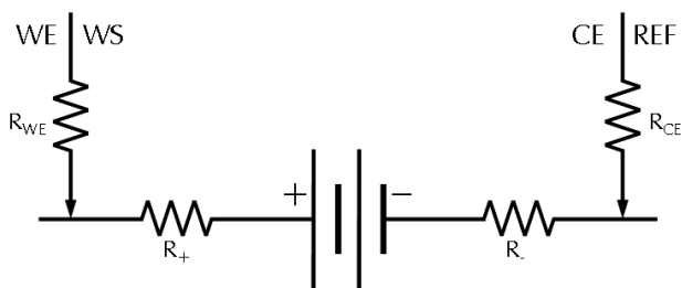
Figure 3. Simplified diagram for a 2-point setup.
