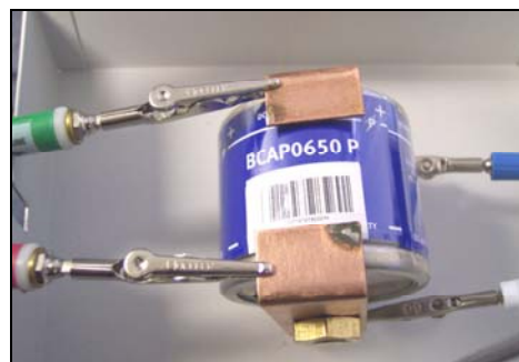
Figure 7 – Electrode connections for measurements on a 650 F EDLC. Working (green), Counter (red), Working sense (blue), and Reference (white).
