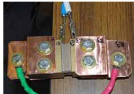
Figure 11 – Fixture and setup for appropriate current distribution and accurate 4-terminal measurements on a shunt
