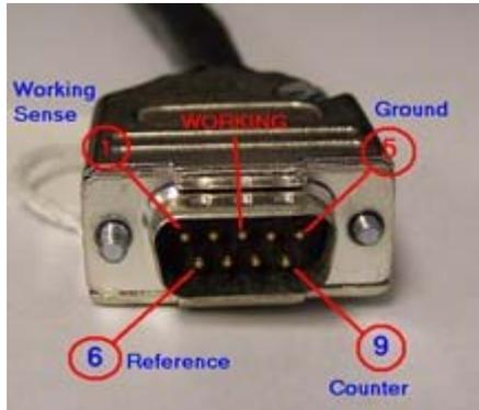
**Pins in the Cell Cable for the Series G, PCI4, PC4 Potentiostats, and ECM8 Multiplexer**
