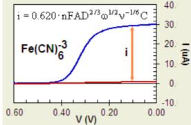
Another consequence of the NDL theory is that the current-voltage curve is S-shaped at scan rates below about 100 mV/s. The limiting current is given by the Levich equation.
