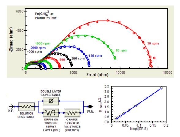
All of the data were fit to the same equivalent circuit model. The plot on the right shows the B parameter of the Porous Bounded Warburg plotted vs. the inverse of the square root of rotation rate. As predicted, there is a nice, linear relationship over two orders of magnitude in rotation rate!
