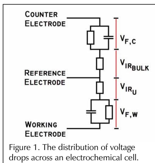
Figure 1. The distribution of voltage drops across an electrochemical cell.
