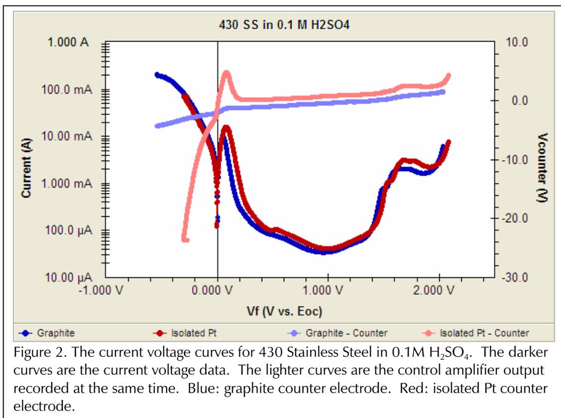
measured current and the slope of the line (  $d\text{Voltage}/d\text{Current}$  ) was about 9 ohms. This represents the total resistance between counter and working electrodes. If we assume that the other three voltage drops in Figure 1 are constant or small, then the resistance of the solution between the working and counter electrodes is 9 ohms or less.
