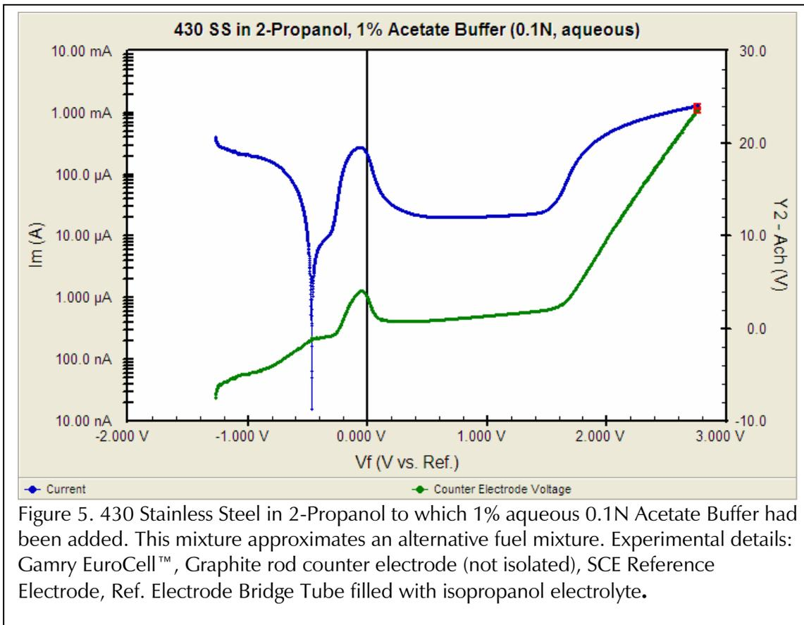
Figure 5. 430 Stainless Steel in 2-Propanol to which 1% aqueous 0.1N Acetate Buffer had been added. This mixture approximates an alternative fuel mixture. Experimental details: Gamry EuroCell™, Graphite rod counter electrode (not isolated), SCE Reference Electrode, Ref. Electrode Bridge Tube filled with isopropanol electrolyte.
