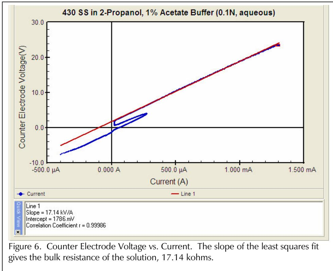
Figure 6. Counter Electrode Voltage vs. Current. The slope of the least squares fit gives the bulk resistance of the solution, 17.14 kohms.
