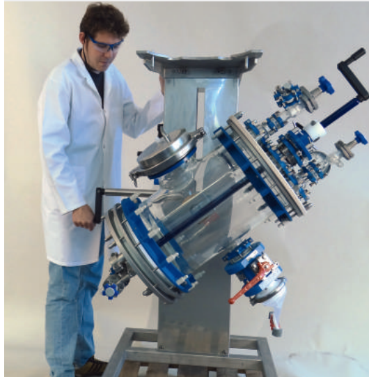
tilting of 30 liter high containment filter vessel for discharge Drehung des 30 Liter high containment Filters für Entladung
